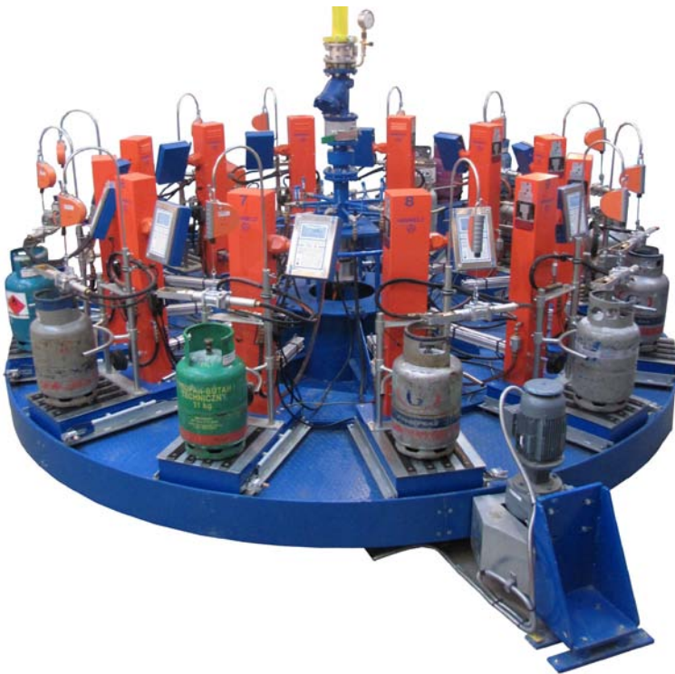
Typical design of a filling carousel
